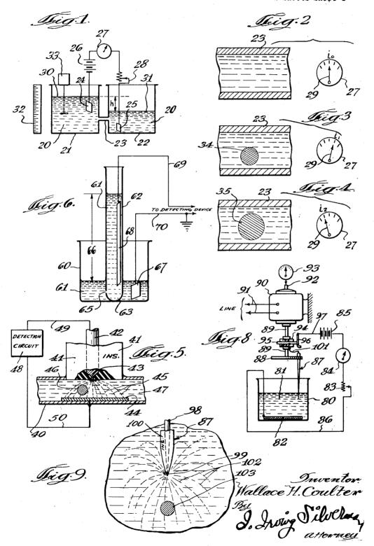
MEANS FOR COUNTING PARTICLES SUSPENDED IN A FLUID
