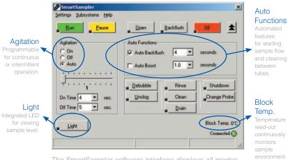
The SmartSampler software interface displays all modes of operation and is easy to use.
